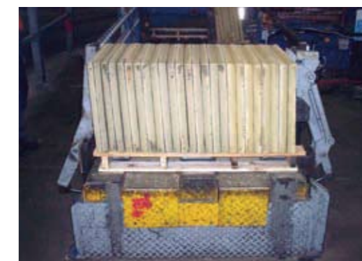
Slabs at the end of the conveyor. Eliminating need to climb onto conveyor and hydraulic arms to straighten slabs.
