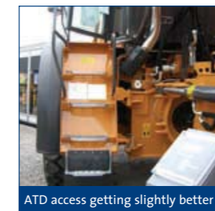
Improving access and guarding for this drill rig
