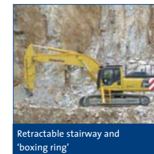
Retractable access – lighting to be added
